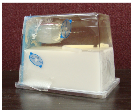
Figure 9-2.1: Ultrasound phantom with brachytherapy seeds.
