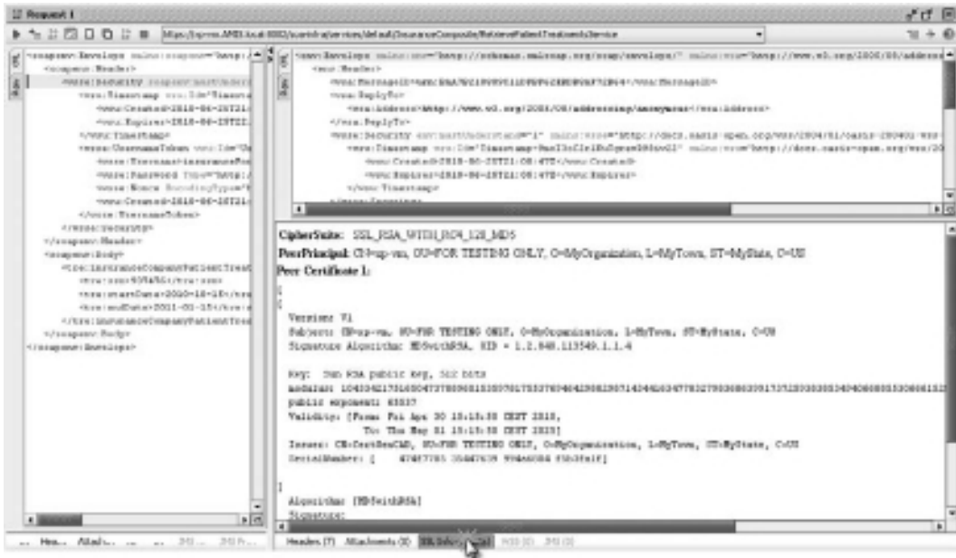
FIGURE 15-22. Inspecting the certificate used to set up the SSL/TLS connection
