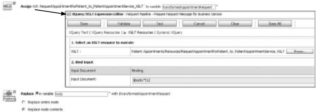
FIGURE 13-20. Configuring the Assign and Replace actions that initialize a variable with the transformed request body and replace the body contents with that variable
