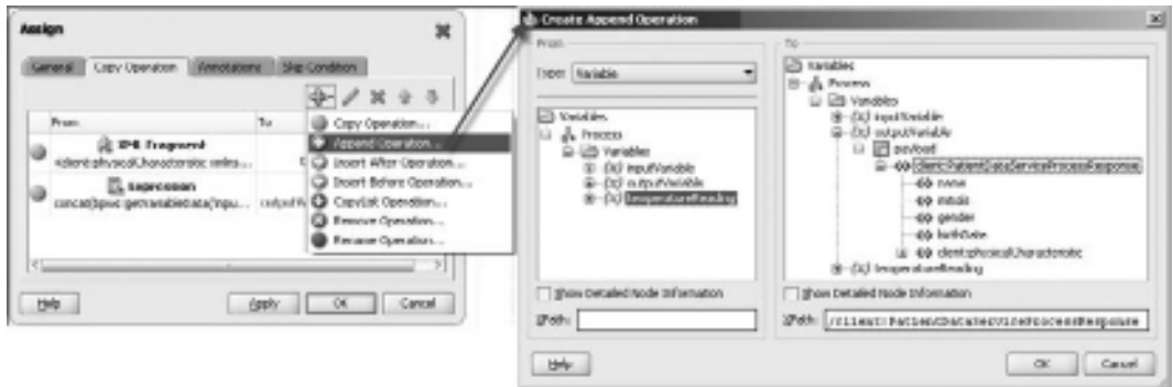
FIGURE 5-9. In the Assign activity, appending the contents of one BPEL variable to a node in another variable
