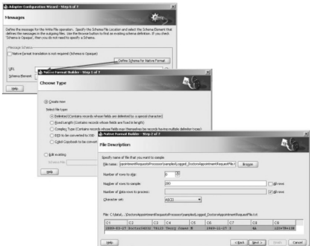
FIGURE 7-3. Using the Native Format Builder to create an XSD for the CSV file format
