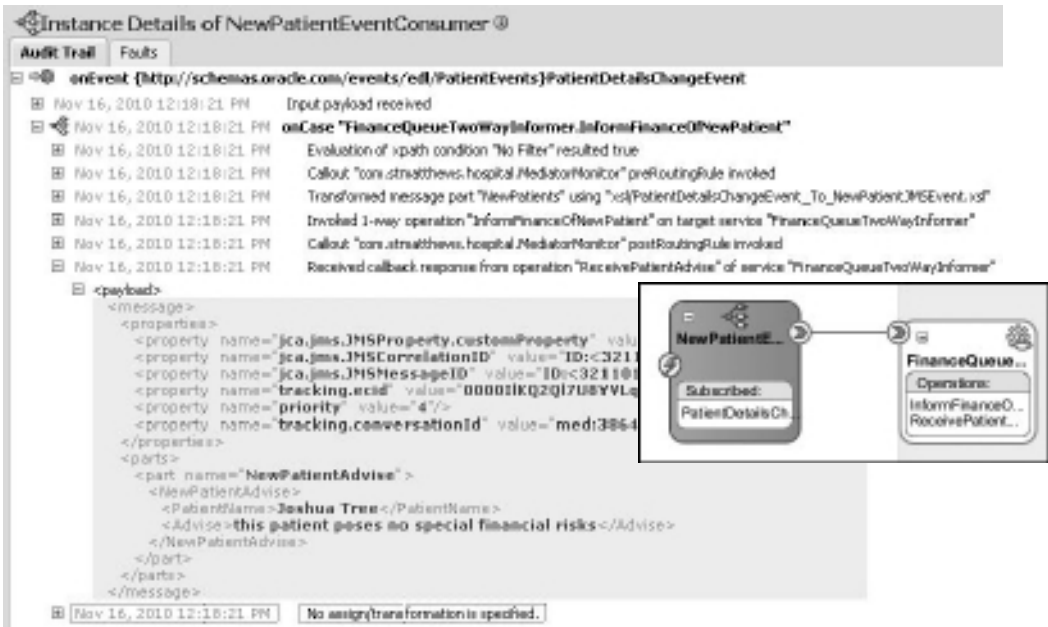
FIGURE 12-8. The two-way request/reply JMS service in action: The Mediator that publishes the new patient event to the JMS adapter service now receives an advise in response.
